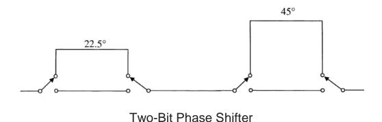
The Phase Shifter in the figure above illustrates an example of a **2-bit Phase Shifter**. Four differential phase states result from switching the four SPDT switches. These differential phases are 0° (reference), 22.5° 45°, and 67.5°. One major application of the multi-bit Phase Shifters is in phased-array antennas.
