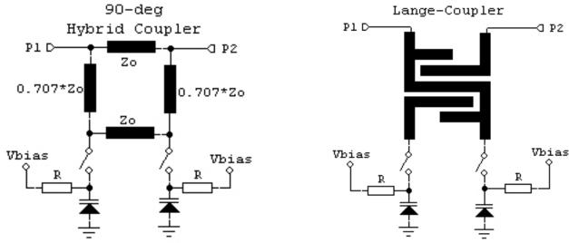
Quadrature Phase Shifters (Hybrid and Lange) using varactors
