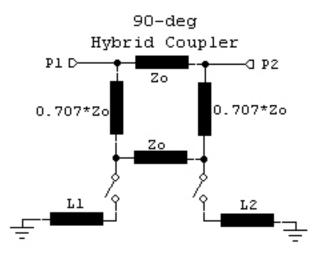
Quadrature Phase Shifter using switched-lines
