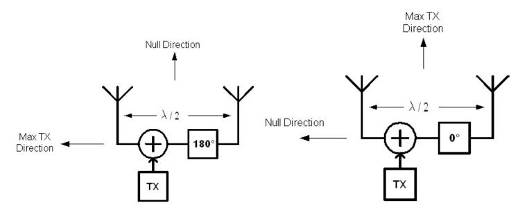
Simple Phase Shift beam forming for Two-Antenna System
