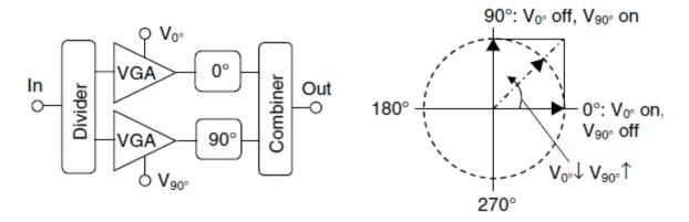
Vector modulation with 90° phase control range and its vector diagram
