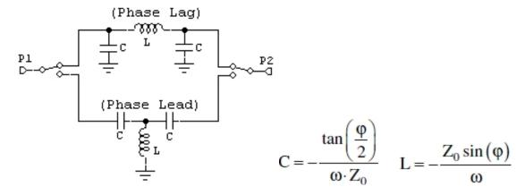
Switched Low-Pass and High-Pass Phase Shifter
