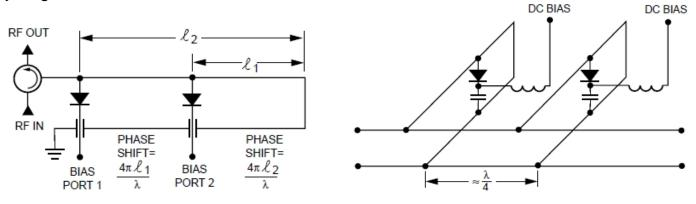
Phase Shifter using Isolator and switched-lines
