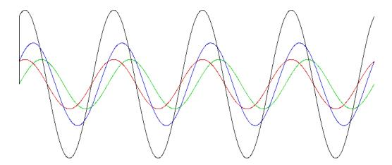
The forward and reflected signal become out of phase, but the cables swr rf signal is still present, stressing the coax insulation materials, the error miss-match voltage signal in black indicating the degree of miss-matched antenna to feedline and radio.
