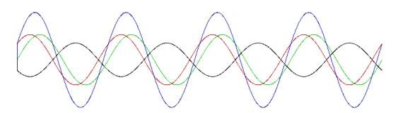
Look to see that the forward and reflected signal are now in a near phase, whereas with an inductive antenna, the forward and reflected signal become out of phase. It is the reflecting and forward phase of the RF signals, that go to stress the coax cabling. Notice the phase signal voltage reversal of the missmatch error voltage between the inductive and capacitive loading.
