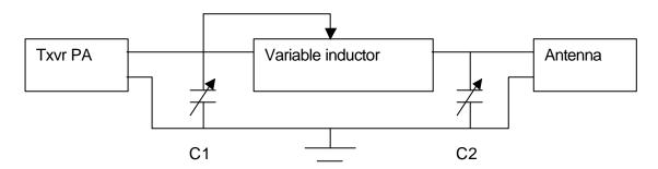
The two capacitors, C1 and C2, act as impedance splitters and conjugate matchers. Imagine the two Cs disconnected from ground – they are now in series and have an L is parallel – ie, we have a parallel LC resonant tank. Our aims are to adjust this tank for
