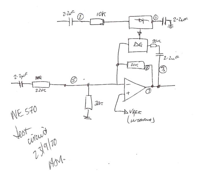
The first test was to determine the through put signal performance without the agc feedback connected.
