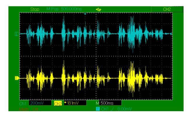
The above diagram plot illustrates the unity gain from the ne570 audio processing circuit. The difference between ch1 and ch2 voltage plot per square, was to calibrate the circuits unity gain signal through put.
