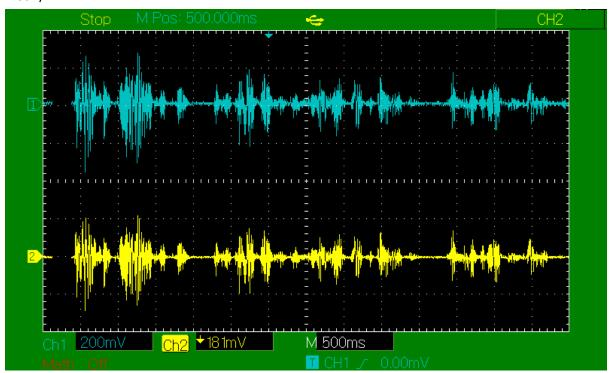
Having compensated for the unity gain value, the audio compression can be clearly seen. Should the agc input connection be instead connected to the circuit output, the following is shown.
